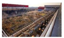
(3) **BIOFILTER** FOR PROCESS AIR TREATMENT
