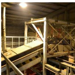
MAGNETIC SEPARATOR TO SEPARATE FERROUS METALS
