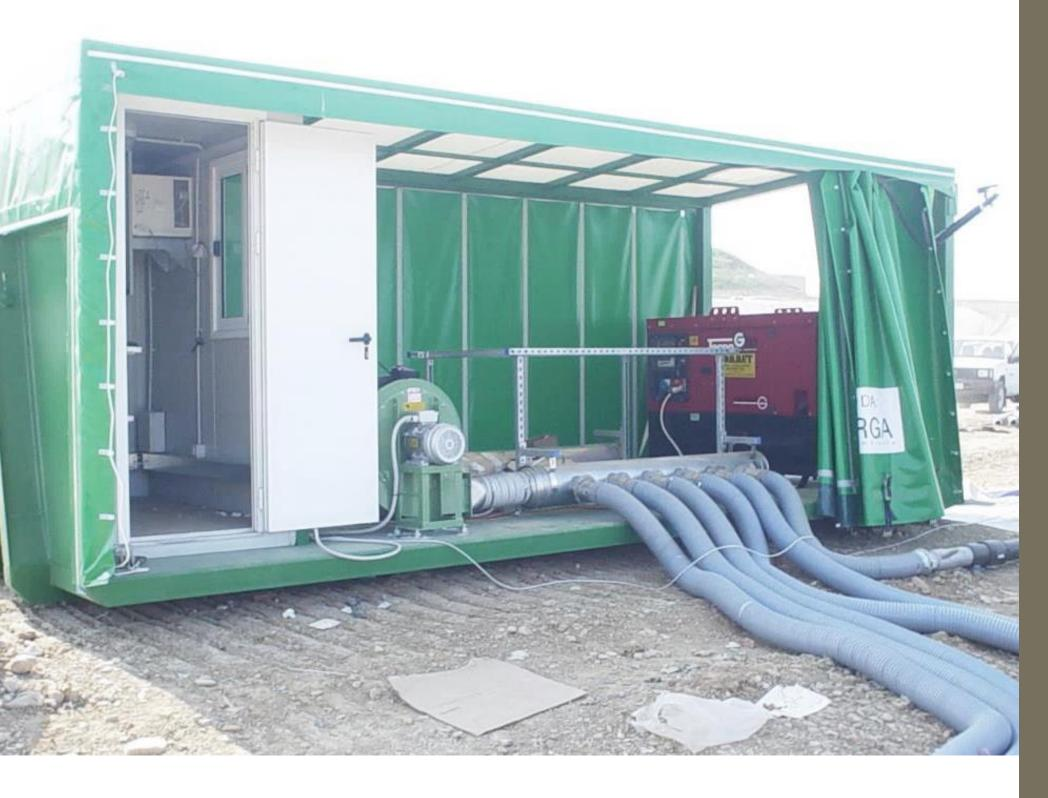
ENTSORGA'S BAT Q-RING ™ IS A **SIMPLE AND MODULAR** DESIGN FOR EFFICIENTLY COMPOSTING ORGANICS OR STABILIZING UNSORTED MUNICIPAL WASTE BEFORE DISPOSAL.
