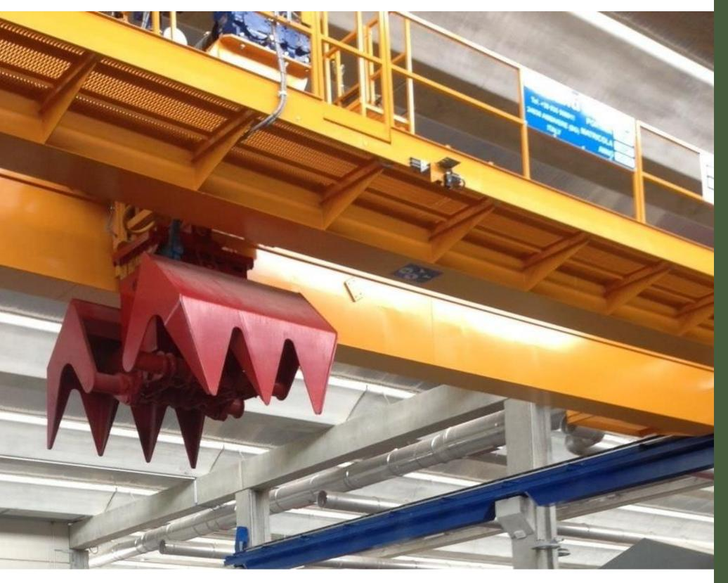
THE **SPIDER™** IS AT THE HEART OF ALL THE ENTSORGA'S HIGH VOLUMES SYSTEMS FOR PROCESSING BULK MATERIAL. **FULLY AUTOMATED HIGH SPEED CRANE** ALLOWS FOR ROBUST AND ENERGY EFFICIENT MATERIAL HANDLING.
