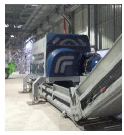
SECONDARY SHREDDER TO ADJUST THE SRF TO THE REQUIRED SIZING
